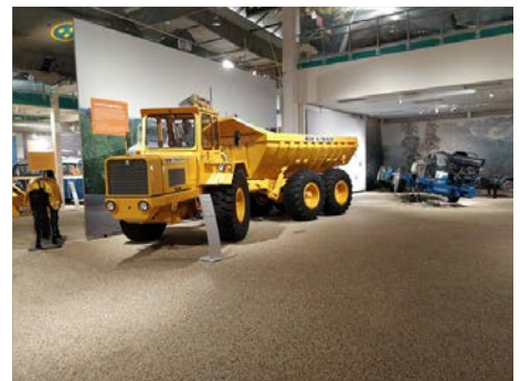
The first model Articulated Hauler based on a farm tractor was developed by BM-VOLVO
