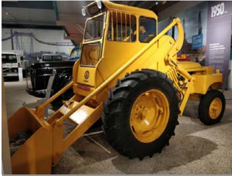
The first Concept Loader built on a farm tractor under the brand of Bolinder Munktell (BM)
